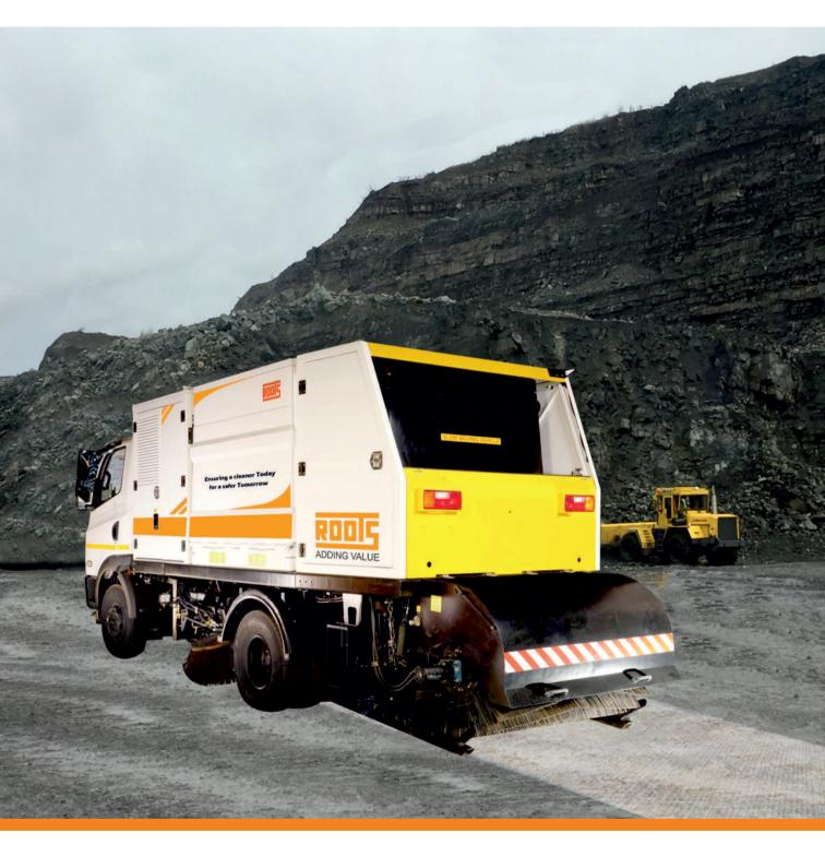
Conveyor Type, Truck Mounted Sweeper with Hopper Capacity of 5 m<sup>3</sup>
