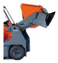
Side broom integrated with the arm - enables riding on bumps and speed breakers easy without any damages.
